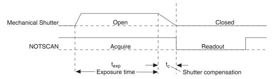
Figure 26. Exposure of the CCD with Shutter Compensation
